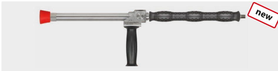
1/4" M. Stainless steel. Longcast lance 350 mm with vented handle ST-29 Cool & Compact 330 mm, grip aside and nozzle protector made out of plastic without nozzle. Max. 280 bar / 130 l/min / 100 °C
