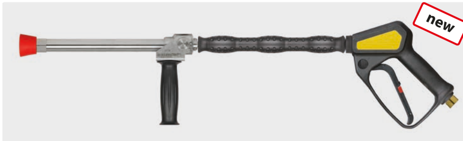
3/8" F. Stainless steel. Longcast lance 350 mm with vented handle ST-29 Cool & Compact 330 mm, gun ST-2300, grip aside and nozzle protector made out of plastic without nozzle. Max. 280 bar / 45 l/min / 100 °C
